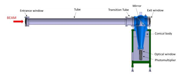
The threshold Cherenkov Detectors (XCET) is a detector used in the Experimental areas at CERN to count the number of selected particles in the beam.
