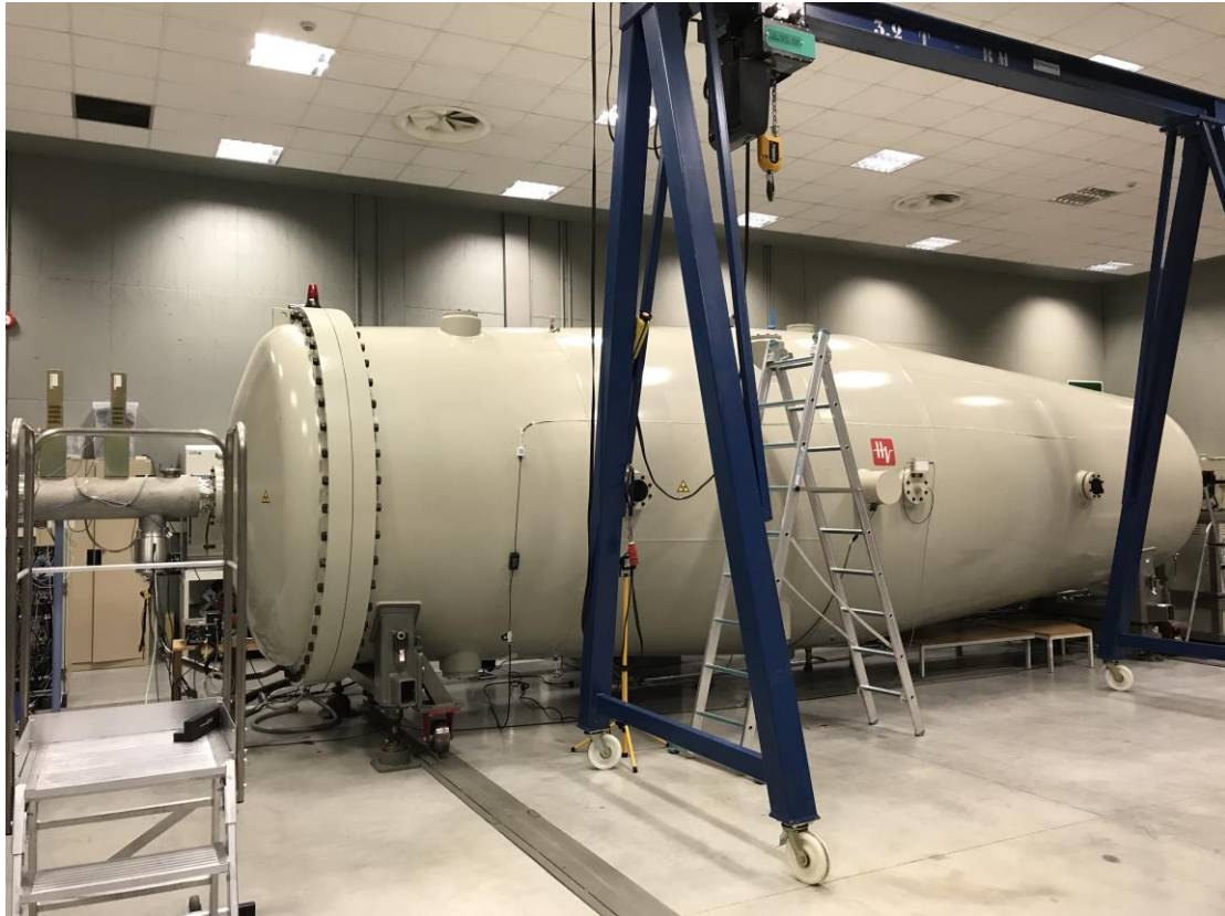
Tandem of 10 MeV at CMAM (Center for Microanalysis of Materials), UAM
