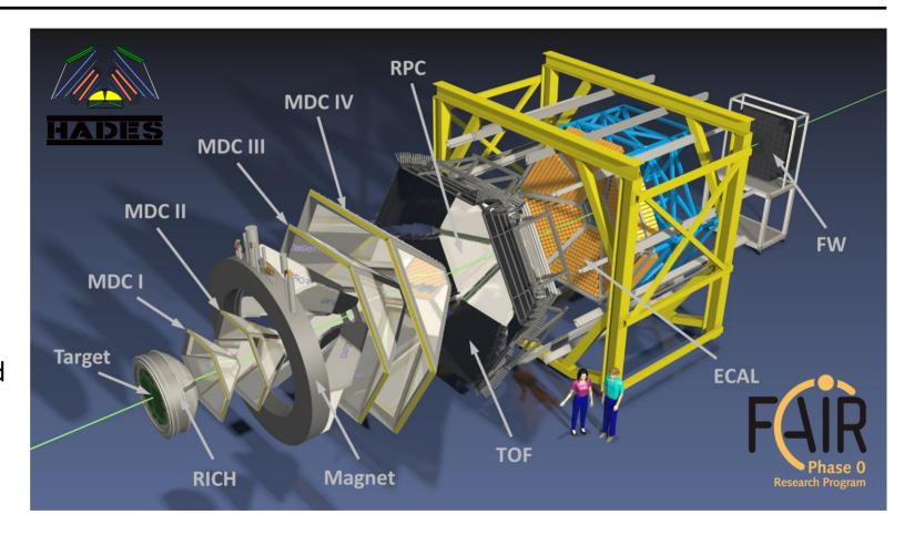
Almost full azimuthal angle and polar angles between 18° and 85° covered
