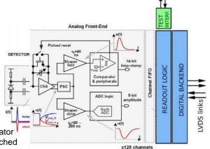
The fact that the chip possesses a double path is not a simple coincidence; this construction allows to establish a more elaborated scheme to suppress the noise keeping a very good time resolution.
