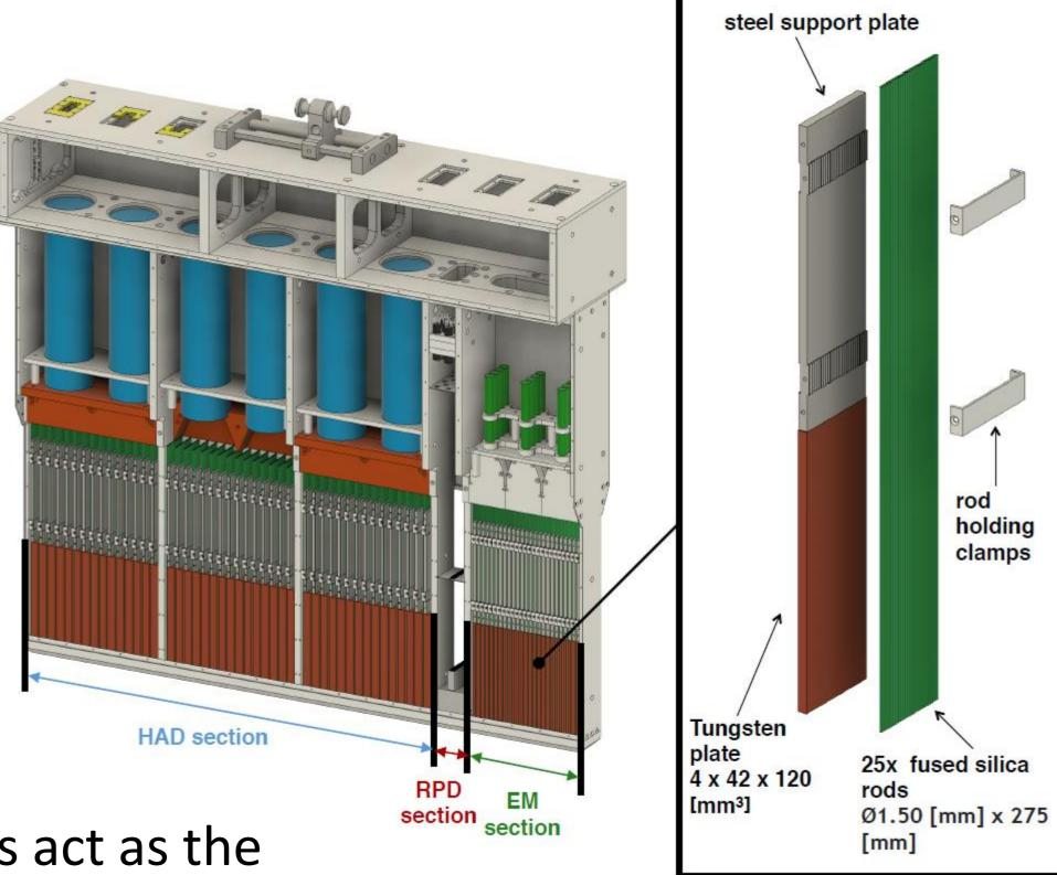
The tungsten plates act as the absorber, creating a particle shower, which in turn creates Cherenkov photons in the fused silica rods that guide the photons upwards towards the PMTs.
