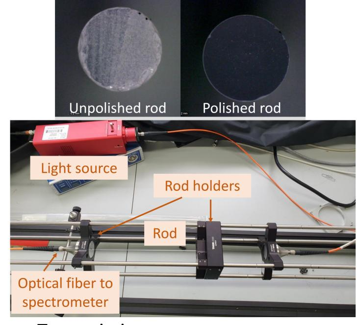
Polishing setup Transmission measurement setup polished (13 rods) JZCaP  $\sigma$  polished \$ 6000  $\sigma$  unpolished Fused quartz (GE124) 5000 Light 9000 19 cm rods 3000 2000 1000 300 350 400 450 500 550 600 650 700 750 800 850 900 950 1000  $\lambda$  [nm]
