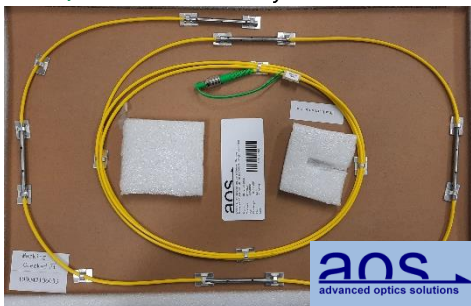
Combined temperature and RH sensors (RHS)
