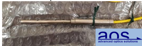
Combined temperature and RH sensors (RHS)
