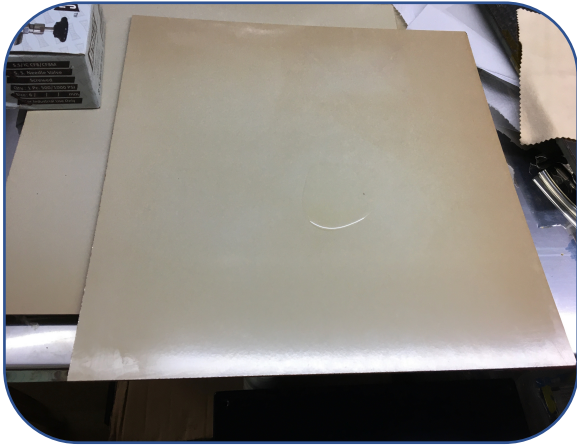
Application of linseed oil on the bakelite surface
