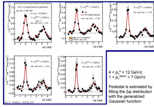
$$f(\Delta\varphi) = b + \frac{\mathbf{Y_{NS}} \times \beta_{NS}}{2\alpha_{NS}\Gamma(1/\beta_{NS})} \times \mathbf{e}^{-(\frac{\Delta\varphi}{\alpha_{NS}})^{\beta_{NS}}} + \frac{\mathbf{Y_{AS}} \times \beta_{AS}}{2\alpha_{AS}\Gamma(1/\beta_{AS})} \times \mathbf{e}^{-(\frac{\Delta\varphi-\pi}{\alpha_{AS}})^{\beta_{AS}}}$$
