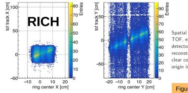
Spatial correlation between tracks from TOF, extrapolated to the RICH detector plane and centers of reconstructed RICH rings. In X and Y a clear correlation with its center in the origin is seen.
