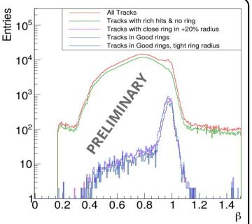
Normalized velocity distribution of tracks formed by 4 hits in the TOF detector. Using the enhancement from electrons and pions at 1 by track-ring matching, the tracks are absolutely calibrated. The comparison to low  $\beta$  range shows the enormous suppression power to protons by the mRICH.
