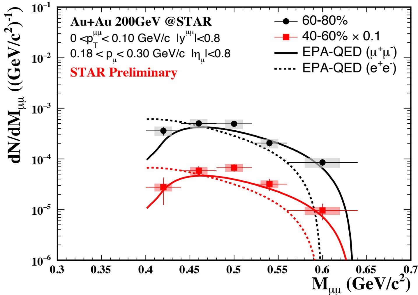
EPA-QED predicts different cross sections due to electron and muon mass difference
