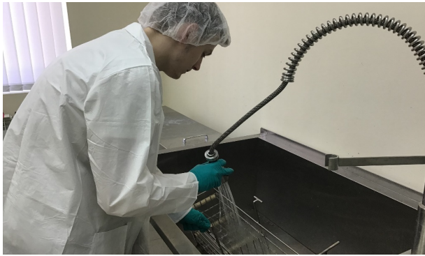
Glass cleaning with ultrasonic wave & deionized water
