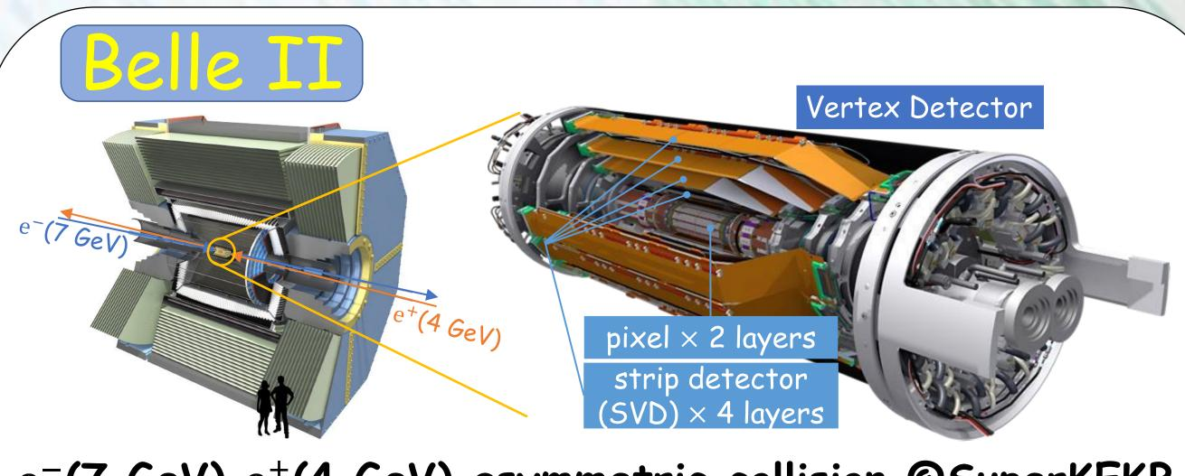
e<sup>-</sup>(7 GeV) e<sup>+</sup>(4 GeV) asymmetric collision @SuperKEKB generate  $B\overline{B}$  and measure lifetime difference by space separation Vertex Detector just outside the beam pipe
