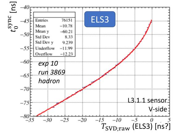
"raw" hit-time is calibrated for each sensor/side to the reference time  $t_0^{\rm sync}$  — event timing estimated by outer detectors offline, called "EventTO" or "TO", synchronized to SVD reference frame.
