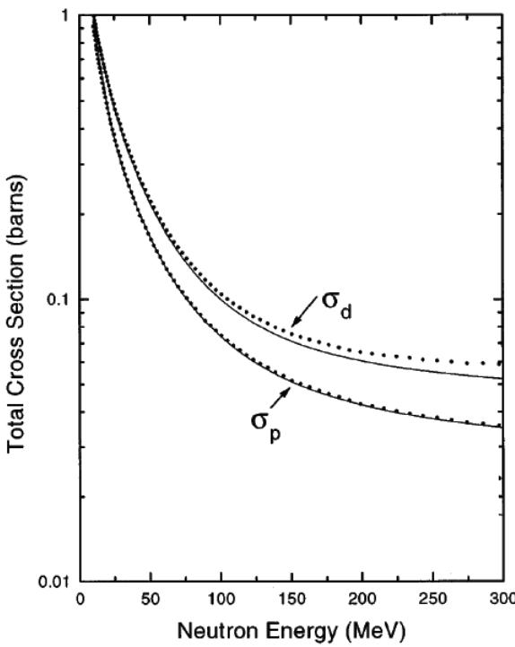
While the NN forces seem under control, large deviations show up for Nd scattering signaling the missing 3N forces
