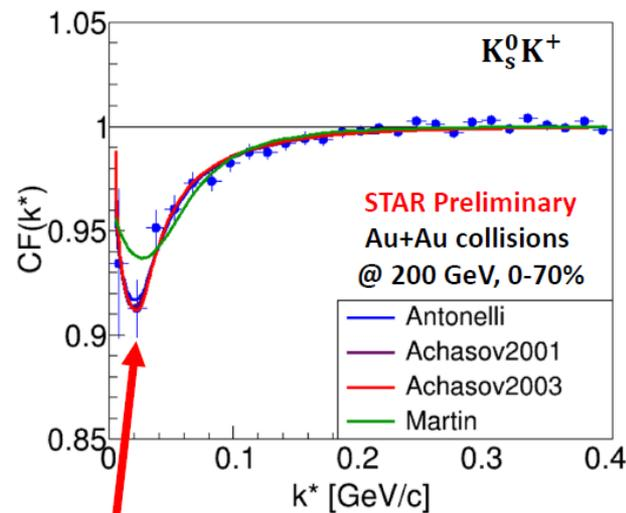
The  $\alpha_0$  FSI parametrization gives an excellent representation of the signal region of the data
