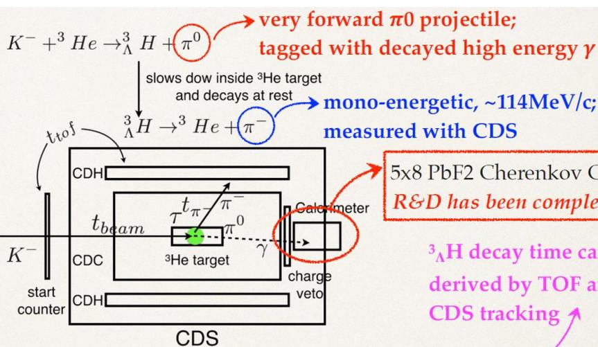
The idea of *direct measurement*:  $T_{\text{CDH}} - T_0 = t_{\text{beam}} + t_{\pi^-} + \tau$
