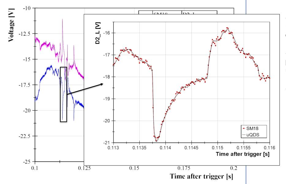
SM18 and uQDS data recorded for the 4.5 K discharge at 9 kA
