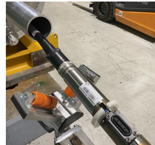
Signal cable connection from Side A
