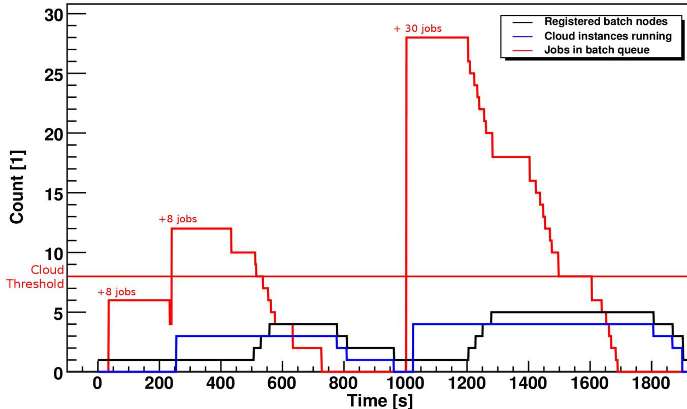
COCCID is able to rapidly increase the computing power of a local PBS by adding Cloud Worker Nodes and adapt to sudden changes in the requirement profile.
