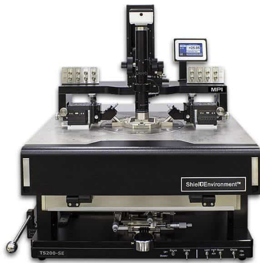
MPI TS200-SE Manual Probe Station with temperature range from -40 to +300°C will arrive soon in Torino Laboratory
