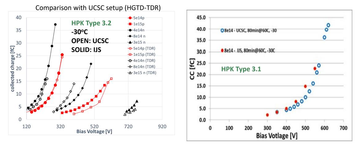
$\geq$  We consider the agreement satisfactory – note that uncertainty in fluence has larger impact for LGADs than for standard detectors due to very high sensitivity of charge collection on V<sub>gl</sub>.
