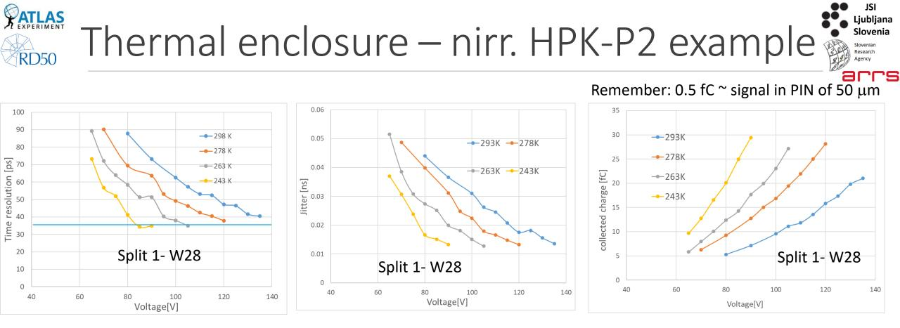
HPK-W28 (V<sub>gl</sub>=54, V<sub>fd</sub>=61 V) -> just enough to reach the desired time resolution and has maximum gain
