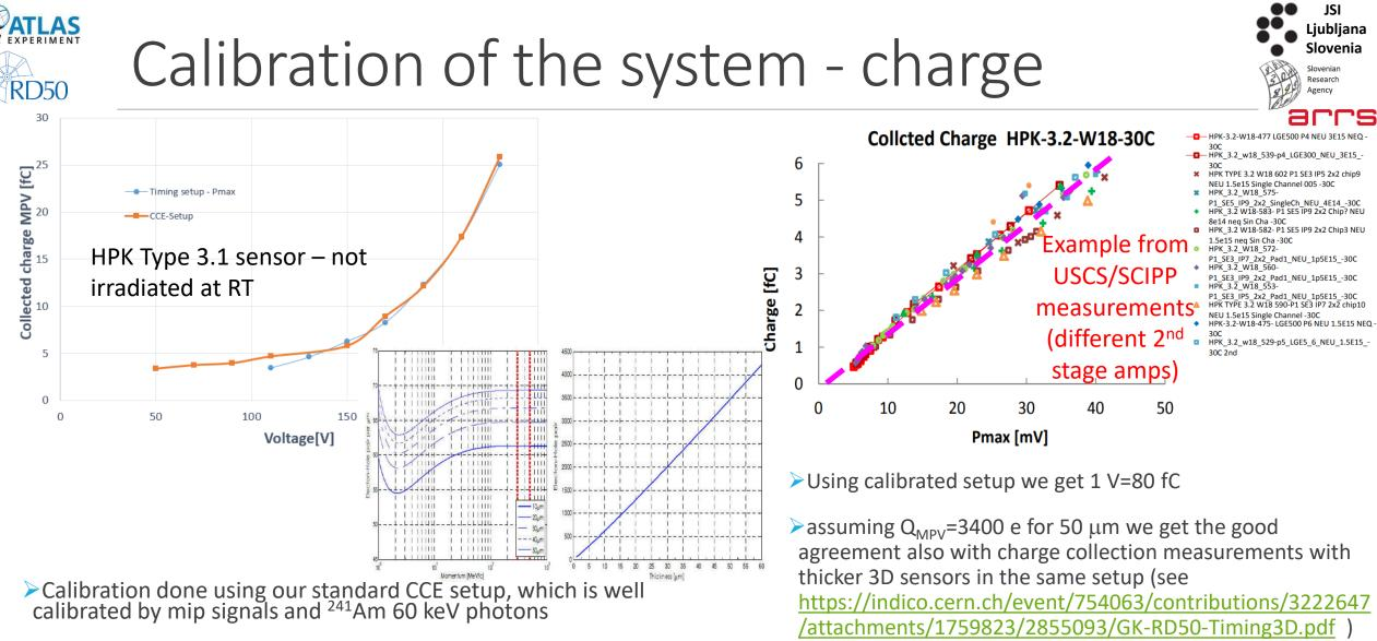
At lower voltages slight disagreement probably due to slower signals and P<sub>max</sub> deviates from integrated charge
