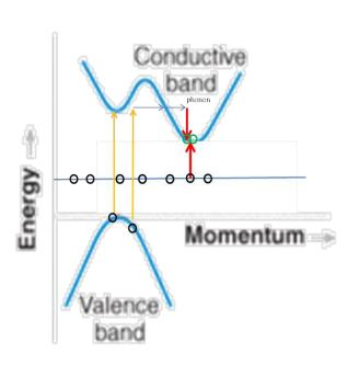
The impact ionization via local levels depends on a density of local level states. (*No restrictions imposed by momentum conservation.*)
