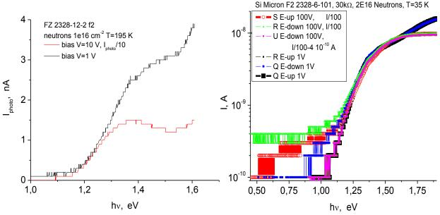
The increase of photo response related to increase of quantum yield started at  $\sim$ 1,4 eV, and due to a decrease of surface passivation by a high bias voltage (our presentation at  $36^{th}$  RD50 Workshop).
