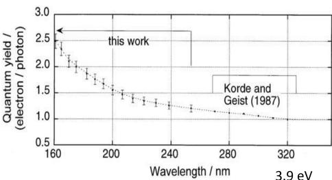
The quantum yield of silicon from 160 nm to 254 nm.R Canfield, R.E Vest, R.Korde et al. Absolute silicon photodiodes for 160 nm to 254 nm photons. (2003) Metrologia 35(4):329
