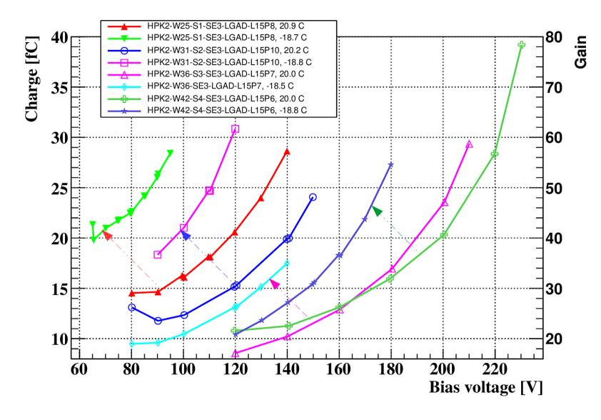
Arrows point from +20 C to -20 C. Measurements in  $\beta$  setup For reference,  $Q_{PiN}$ =0.5 fC Note: charge values are mean values of charge distributions
