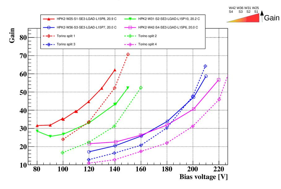
~25% gain differences wrt Torino measurements (to be followed up) We use mean value to calculate charge.
