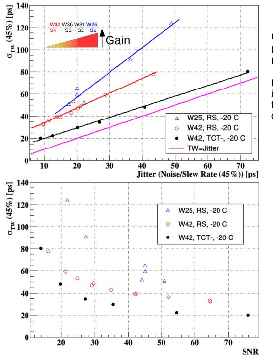
Time resolution after TW correction always better in TCT than in RS because of absence of Landau noise in the rising edge of the pulse.
