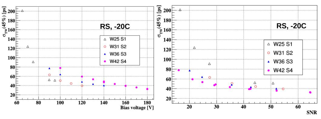
Best timing resolution (30 ps) with RS achieved with W42 (lower gain split) at -20 C, 180 V.
