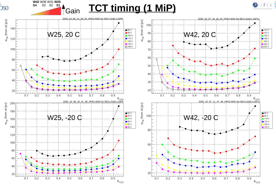
• Timing with laser measured using a direct and +50 ns delayed copy of the original pulse (see backup). Beam **focused** ( $\sigma \sim 10 \ \mu$ m) on the center of laser window
