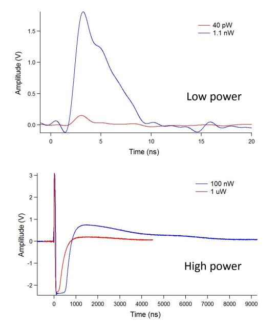
Maximal achievable bias is 400 V but at this value there is no pulsed signal (just noise). **To see clear pulse we**
