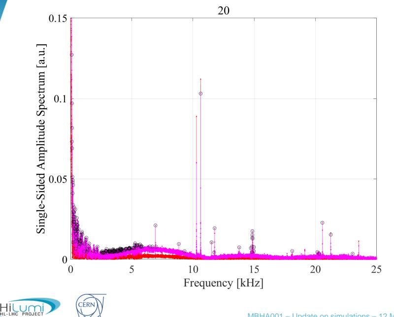
FFT of D1L+D2L – 11.85 kA – QH of D1U delayed
