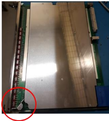
Special design to drive air mostly through the dissipating part
