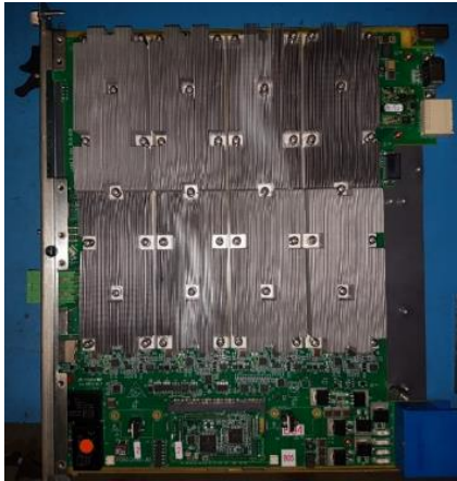
Heat sinks close to the face of the board, lack of air duct
