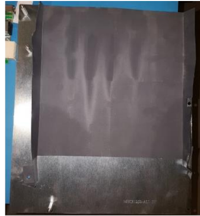
Heat sinks close to the face of the board, lack of air duct
