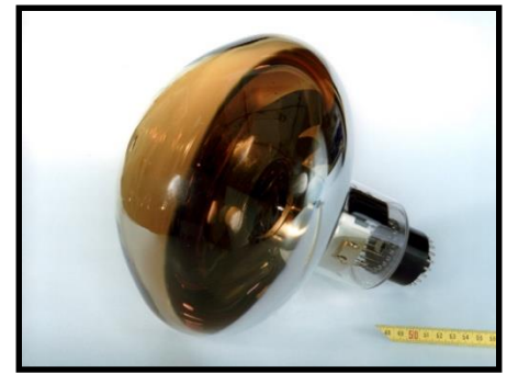
Hamamatsu PMT : Size :10 inch
