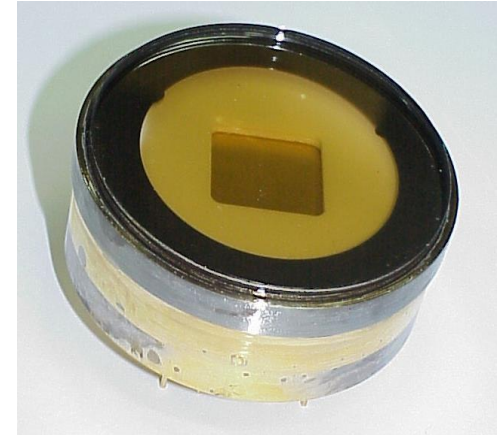
GEM with semi-transparent Photocathode (K-Cs-Sb)
