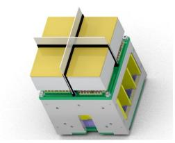
Mechanically stable, cooled and easy to maintain. In total 1052 ECs for both RICHes (122880 channels only in RICH1).
