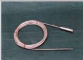
Fission Detector with MI cable for Source Range Monitoring ( BWR)
