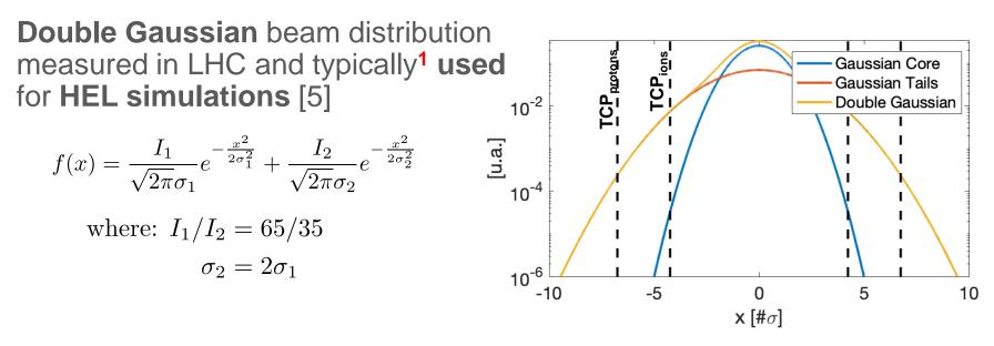
• **TCP aperture** 5.7 $\sigma$  (wrt  $\epsilon_N$  = 3.5 µm) equal (in mm) for protons and ions
