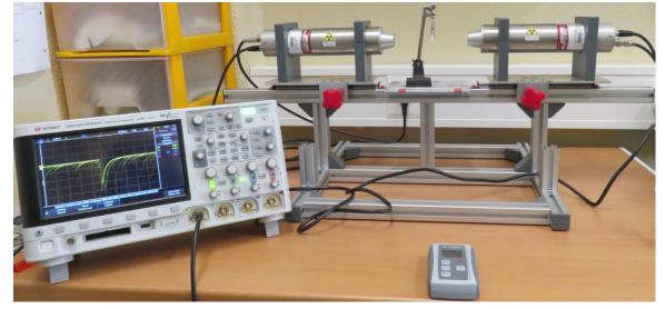
The time difference between the two signals gives the *positron lifetime*.
