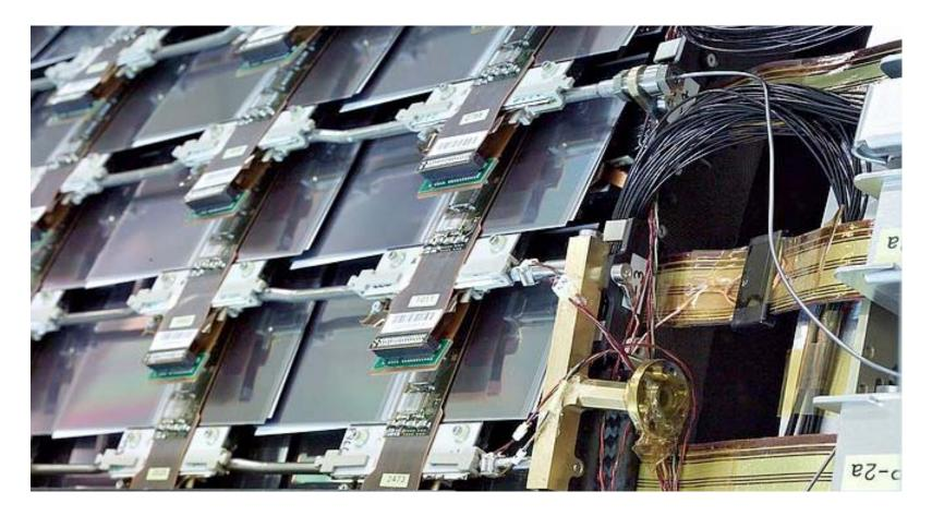
80 µm strip pitch (125 per mm) 6 M channels
