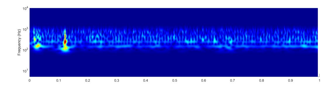
Coil voltage: reconstruction after filtering [100 1000] Hz
