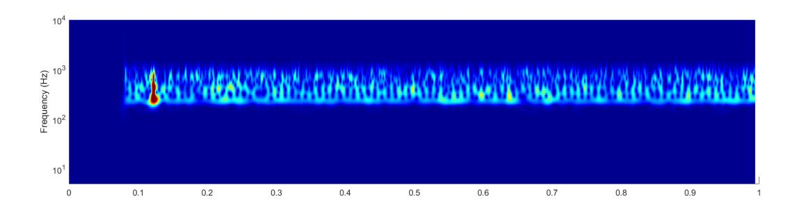
Coil voltage: reconstruction after filtering [100 200] Hz
