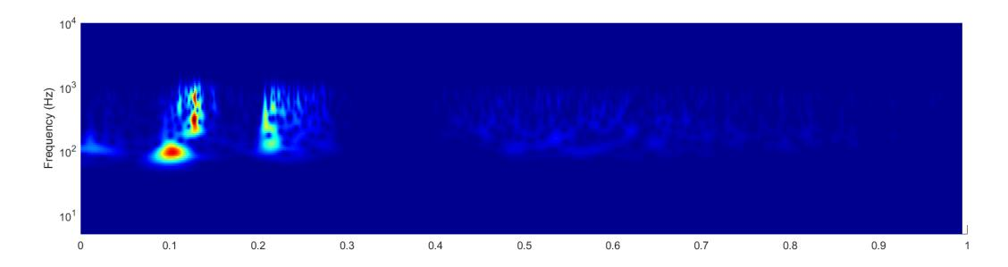
Aperture voltage: reconstruction after filtering [100 1000] Hz
