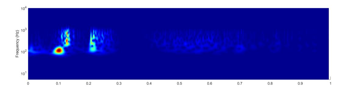
Coil voltage: reconstruction after filtering [100 1000] Hz
