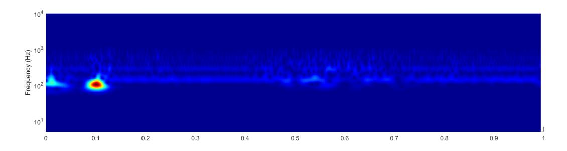
V sum: reconstruction after filtering [100 1000] Hz
