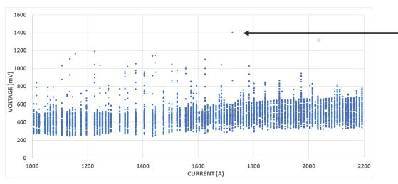
1400 mV spike at 1724 A during a 6000 A ramp
