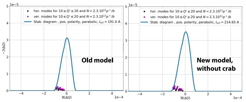
$\Rightarrow$  The impact on stability is ~13% -- the increase of tune shifts for the most critical plane (horizontal) is lower than for the other one.
