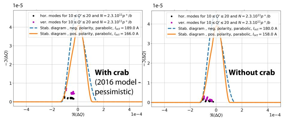
⇒ Despite a quite significant effect on imaginary tune shifts, the impact of crab cavities on stability is small (<10A, i.e. 5%) – note that here, **teleindex~2** as the v1.4 optics with  $\beta^*$ =40cm are used.
