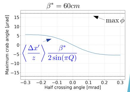
> A crab angle of maximum 5 µrad can be expected due to the crossing angle
