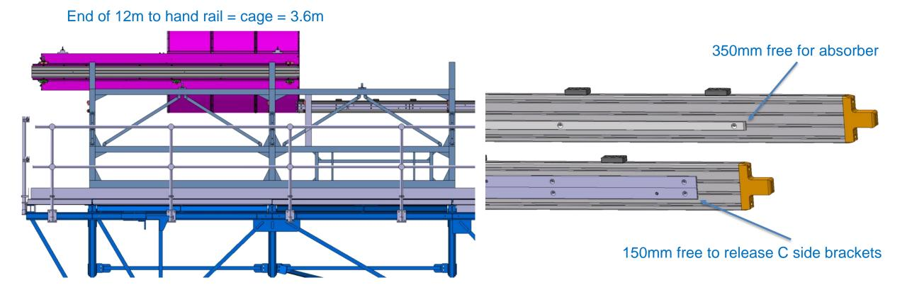
cage lowering: last temp rails section holded in C beam, ST1311703\_01 design ongoing
