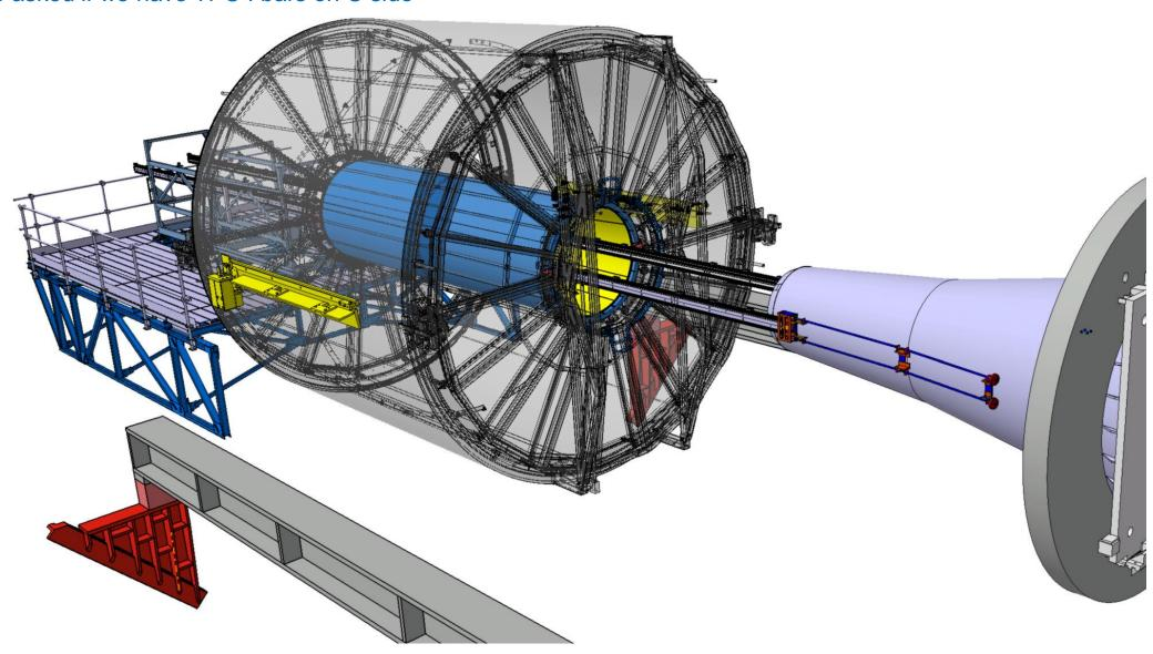
**Beam pipe :** cad assembly modified to match installation process, beam pipe + valve + trolley
