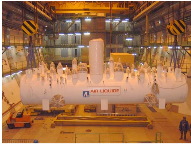
Cryogenic interconnection box
