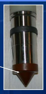
Fiber Glass Stem for low heat inleak
