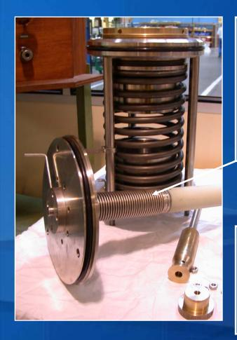
Bellows sealed type for better tightness (double bellows type for QV valves)
