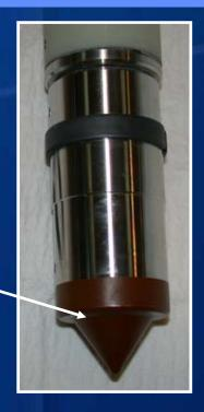
Fiber Glass Stem for low heat inleak
