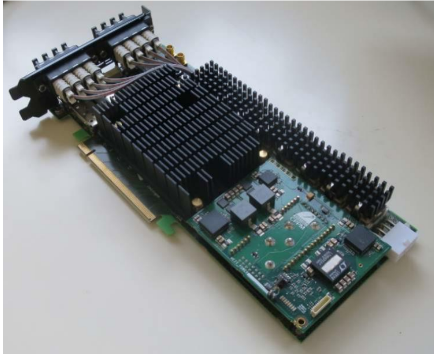
PCIe40 card (so-called TELL40) Up to 48 optical links
