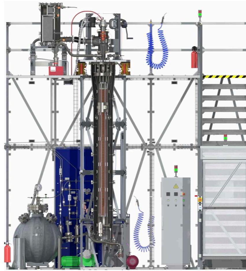
Test e- drift over 2.6 m (purification, high-voltage)
