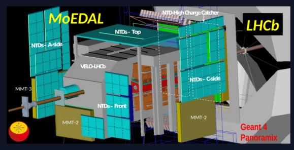
Analysis of the NTD uses an etching and scanning procedure to search for any HIP tracks in the material, while the MMT material is analyzed using a SQUID magnetometer.
