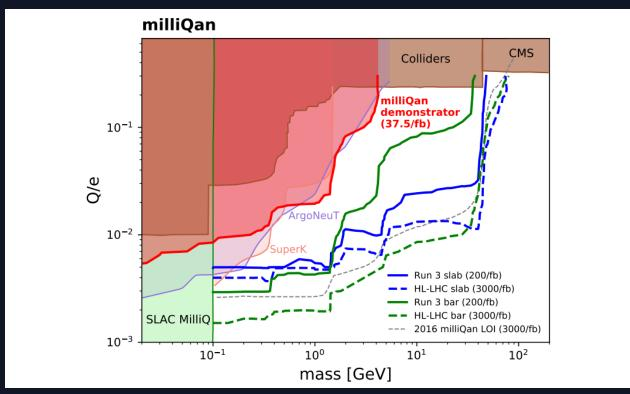
N.B. The HL-LHC projections also include improvements to the milliQan detector, such as an increased number of scintillator bars in each layer of the bar detector and an improved active veto, thus reducing the total BG.
