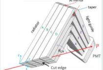
Far stations consist of two subdetectors: Silicon Tracker (SiT) and ToF detector. Time-of-Flight (ToF) system is used to reduce the background from multiple proton-proton collisions; it has an "L-shape" and consists of several parts: radiator - light guide - photomultiplier - back-end electronics.
