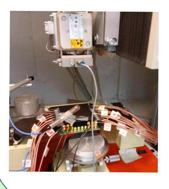
Farmer Chamber dose/Si dose ratio was evaluated in the Padova INFN x-ray irradiation station comparing the PTW dose read-out against the read-out of the CERN calibrated diode for Si dose measurement during a specific irradiation session, performed in March 2021, using the planed SiPM radiation field.
