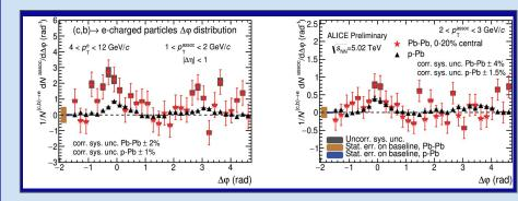
Enhancement observed at near-side peak in Pb-Pb compared to p-Pb, although the large uncertainties in Pb-Pb analysis do not allow for a firm conclusion.
