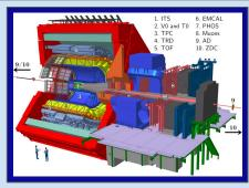
> Electromagnetic calorimeter (EMCal):  $|\eta| < 0.7, 80^{\circ} < \varphi < 187^{\circ}.$
