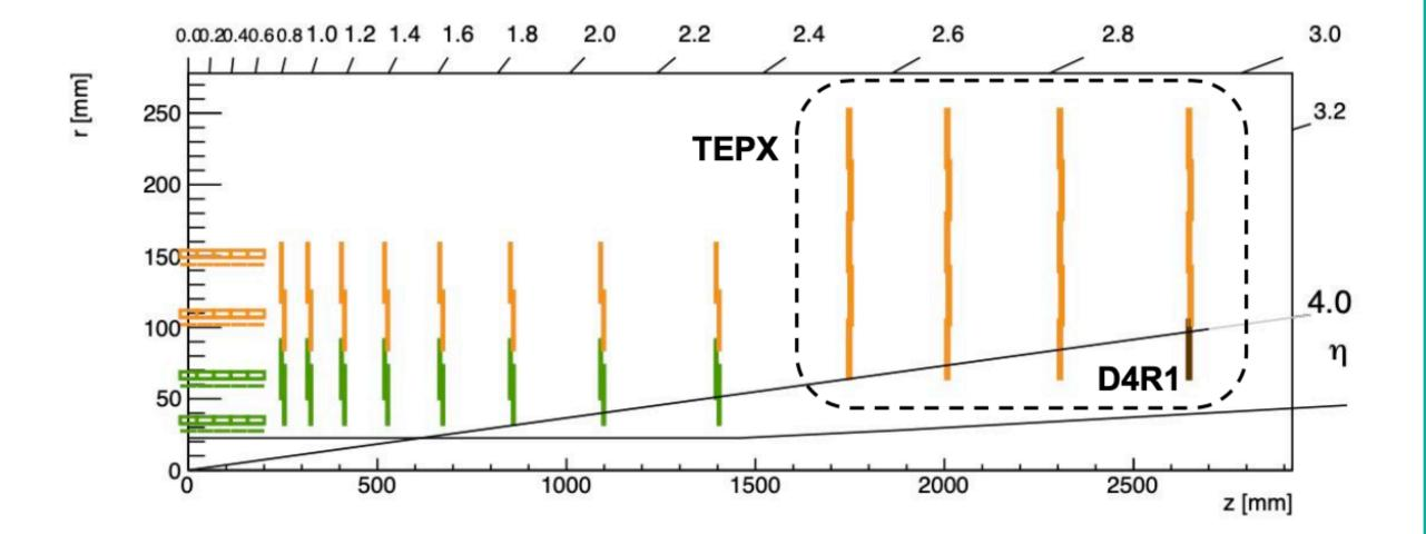
TEPX is planned to be used by BRIL as an independent luminosity and Beam-Induced Background (**BIB**) detector in LHC Phase 2, with the following properties:
