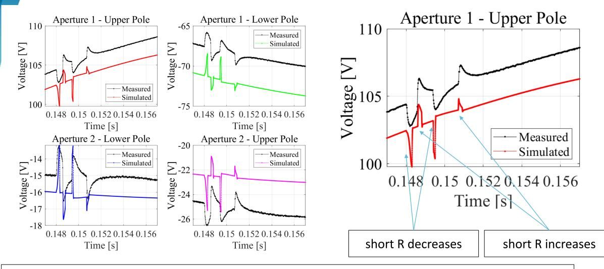
• The change of the voltage spike polarities is likely caused by the change of the short circuit resistance (short appearance / "disappearance")
