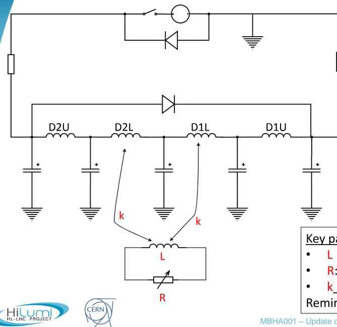
Sudden magnetic flux variation is modeled as a sudden increase/decrease of the RL loop resistance:  $U_{spike} = d\phi/dt = M^* dI_{loop}/dt$  $= k^* sqrt(L_{coil}^*L)^* dI_{loop}/dt$
