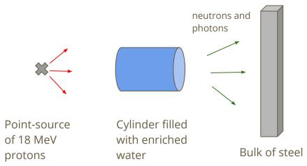
F4 tally: neutron (or photon) fluence averaged over the volume of the bulk (in 1 / cm<sup>2</sup>):
