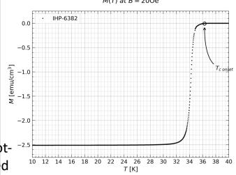
$3^{rd}$  run of samples: MgB<sub>2</sub> specimen made by RHP prepared by hotpressing synthesized powders. Up to 10 layers of MgB<sub>2</sub> deposited by plasma spray on Cu and Al<sub>2</sub>O<sub>3</sub> substrates. The latter have not shown good results due to background noise.
