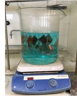
SUBU and Electropolishing treatments Courtesy of E. Chyhyrynets and C. Pira (INFN)
