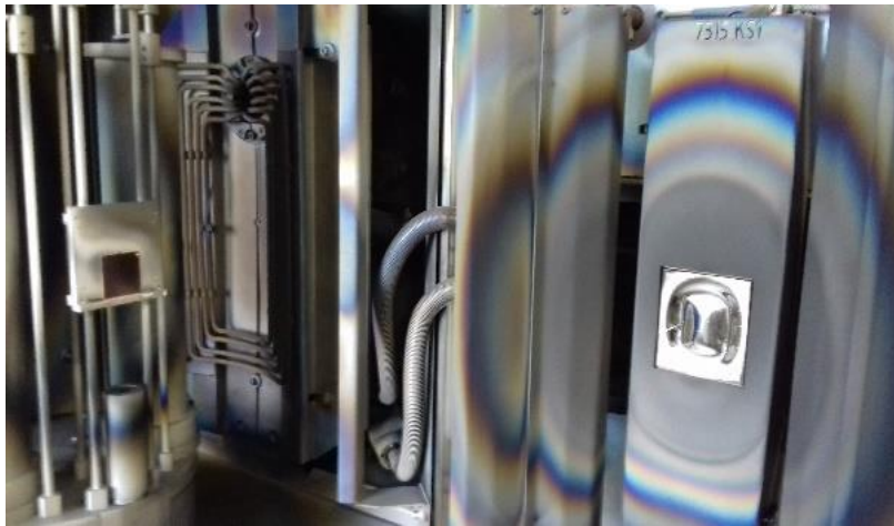
A sample and a Nb target in deposition facility at University Siegen. Courtesy of M. Vogel (Siegen)
