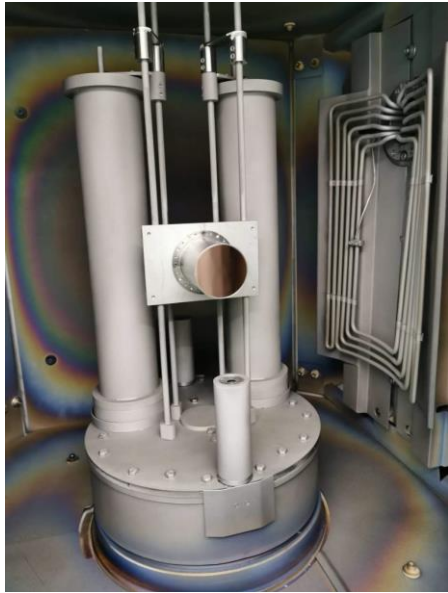
A QPR sample inside the deposition chamber at Siegen Uni. Courtesy of M. Vogel
