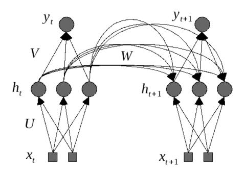
Two input, three hidden nodes. Unfolded one time step!
