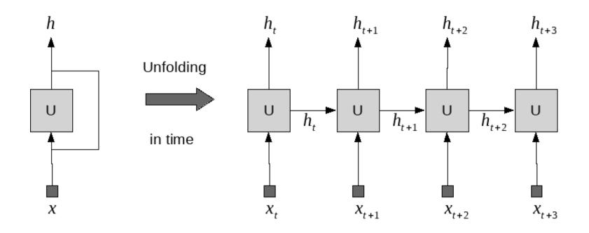
For a LSTM network we simply replace the "U" box with a LSTM box and add a new connection,
