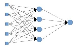
**MLP:** 5 inputs, 4 hidden nodes, a single linear output node.
